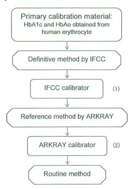
IFCC calibrator (1) is assigned using the Primary calibration material and Definitive method by IFCC. The Reference method by ARKRAY is calibrated by IFCC calibrator (1). IFCC value of ARKRAY calibrator (2) is assigned using the Reference method by ARKRAY.
